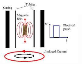
The MTD Tools works on the Pulsed Eddy Current (PEC) principle, which is a broadband Electromagnetic transmitted signal which sets up on eddy current flowing in the external tubular(s).
